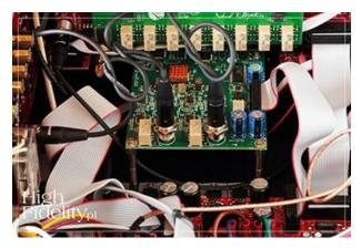
The digital inputs for the audio signal are part of a D/A converter. On the other hand, the **LAN port is an input of a files transport**, which together with
