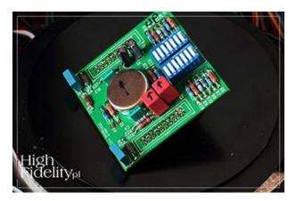
The second card adds DIGITAL INPUTS to the functionality of the device and one of an AUDIO FILE PLAYER. It is a card that is plugged in from the outside (the phono stage is plugged in), which offers three digital inputs for the audio signal -RCA, Toslink and USB - and one digital input for audio files - LAN (RJ45). RCA and Toslink inputs accept PCM signal up to 24/192, and the **USB adds support for DSD signal from DSD64 to DSD256** (11.4 MHz).
